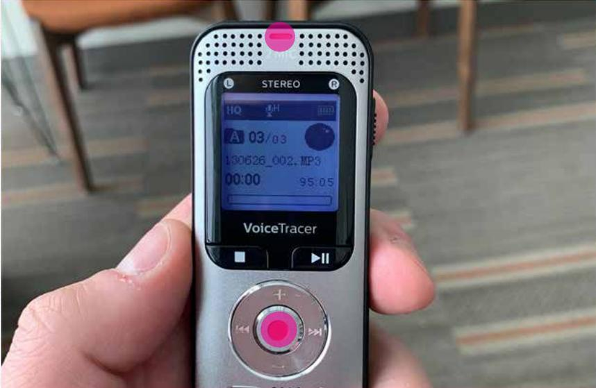
When you are finished recording, press the stop button. The red recording light will shut off.
